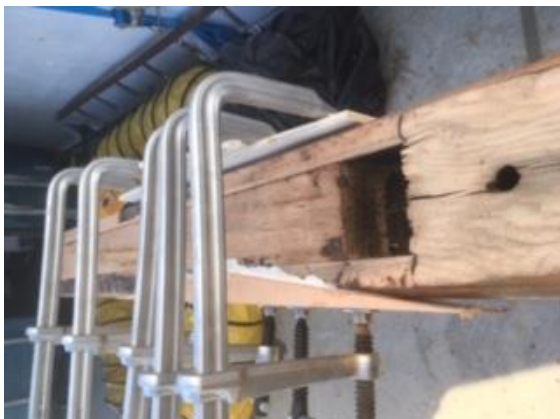
Old hahogany margine plank chizelled out to conserve the plywood underneath.
