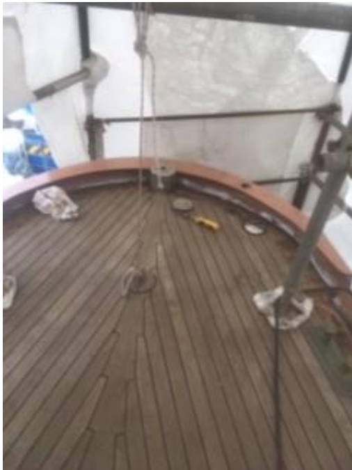
Old hahogany margine plank chizelled out to conserve the plywood underneath.
