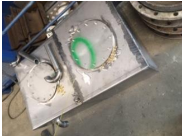
New Black water and grey water tanks after fabrication.
