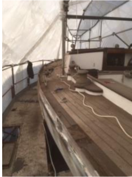
The teak on the inner and outer side of the capping rail came off and the corrosion was treated properly with sandblasting and corroless paint.
